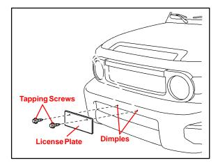
Use self-tapping screws of a non-corroding type with the following dimensions:
